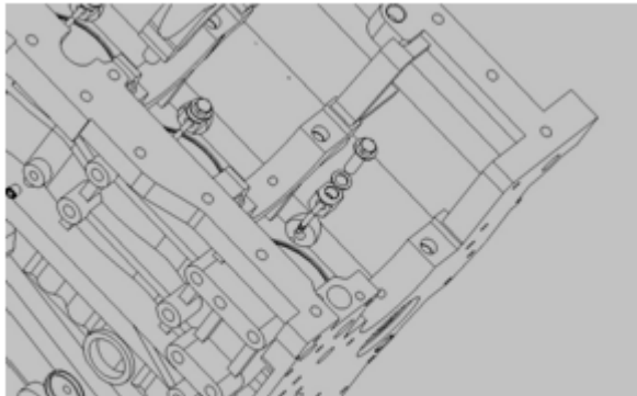
图 2-13 活塞的润滑油冷却喷钩 Fig 2-13 Lubricating oil cooling injection hook
