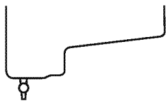
Drain valve installation by lowering the bottom by one step
