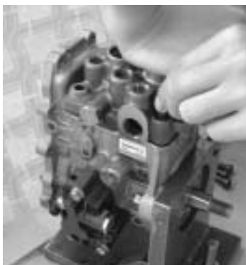
Install the hydraulic head CMP.
