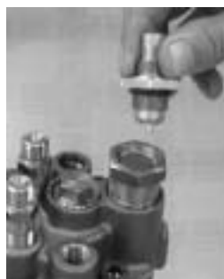
Install the thermo-element with new O-ring.
