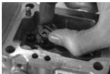
Remove the joint, (distribution shaft).
