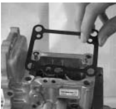
Remove the packing.
