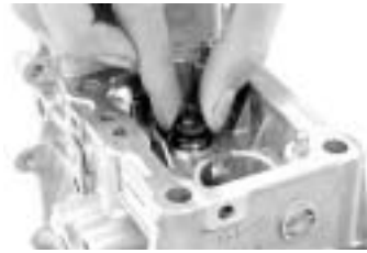
Lift the transmission shaft slightly by your hand.
