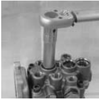
Fasten the plug, (distribution shaft).
