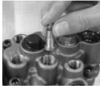
Install the delivery valve CMP.
