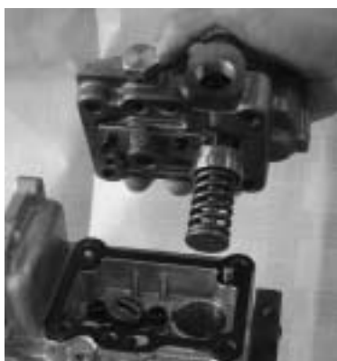
Remove the hydraulic head CMP.
