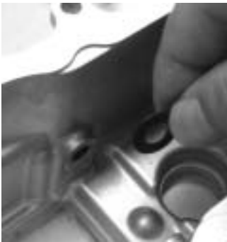
Governor Lever CMP End Float Adjust Shim
