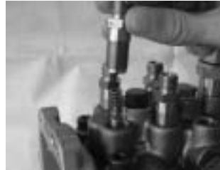
Remove the delivery valve and gasket.
