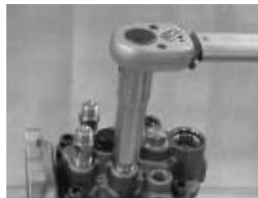
Install the holder, (delivery).
