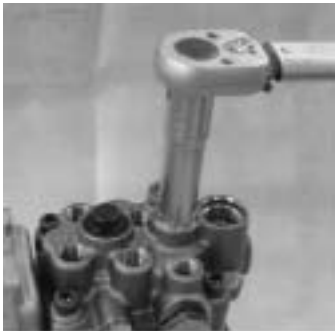
Fasten the plug, (barrel).
