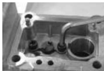
Remove the removal stop, (transmission shaft) fastening bolt.
