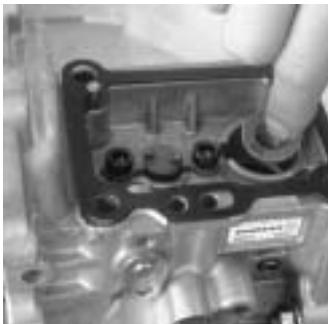
Assemble the FIC adjust shim inside the tappet.
