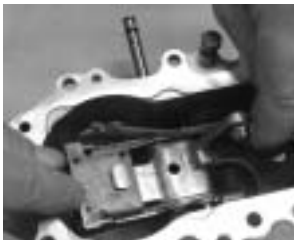
Governor Lever CMP End Float Adjust Shim
