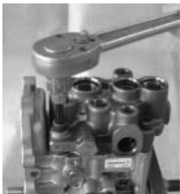
Remove the hydraulic head CMP fixing bolt.
