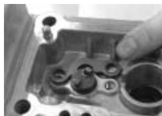
Remove the removal stop, (transmission shaft) fastening bolt.
