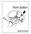
(1) If you press the button on the top of the multifunction switch, the horn will sound.
