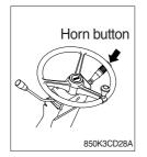
(1) If you press the button on the top of the multifunction switch, the horn will sound.
