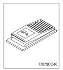
(1) This switch use to operate the front and rear work lamps by two step.
