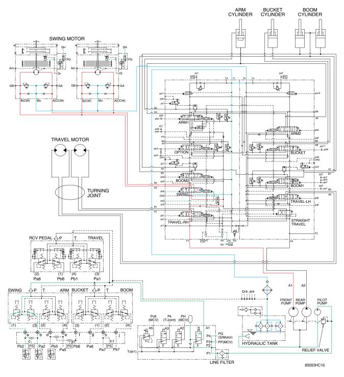
When the LH control lever is pushed left or right, the swing spool in the main control valve is moved to the left or right swing position by the pilot oil pressure from the remote control valve.
