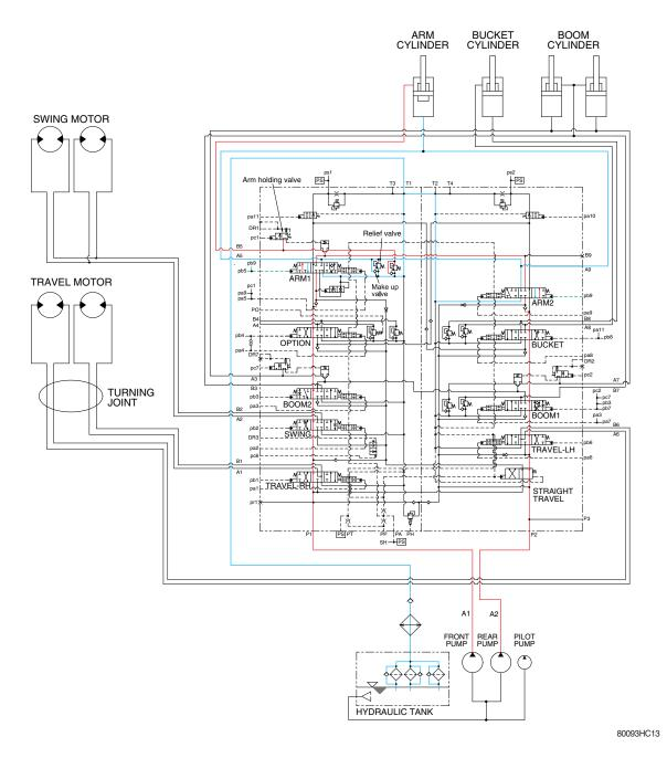
When the LH control lever is pushed forward, the arm spools in the main control valve are moved to the roll out position by the pilot oil pressure from the remote control valve.
