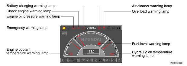
\* Each warning lamp on the top of the LCD pops up on the center of LCD and the buzzer sounds when the each warning is happened. The pop-up warning lamp moves to the original position and blinks when the select switch is pushed. And the buzzer stops. Refer to page 5-41 for the select switch.
