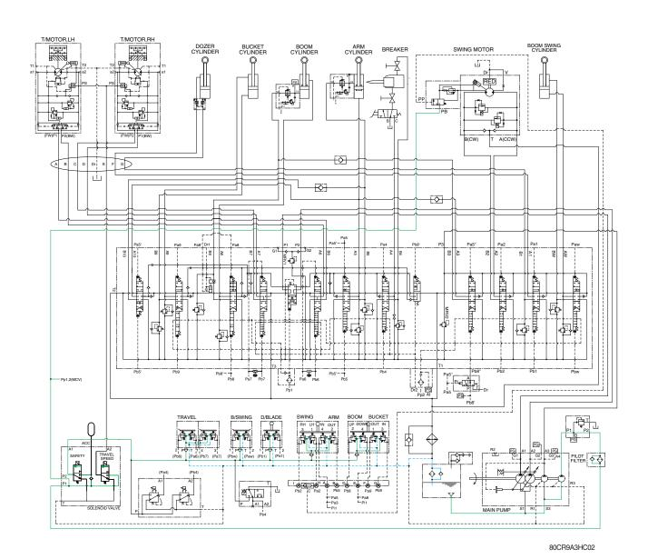
The pilot pump receive oil from the hydraulic tank. The discharged oil from the pilot pump flows to the safety solenoid valve through the line filter. The oil is filtered by the line filter. The pilot relief valve is provided in the pilot pump for limiting the pilot circuit pressure.
