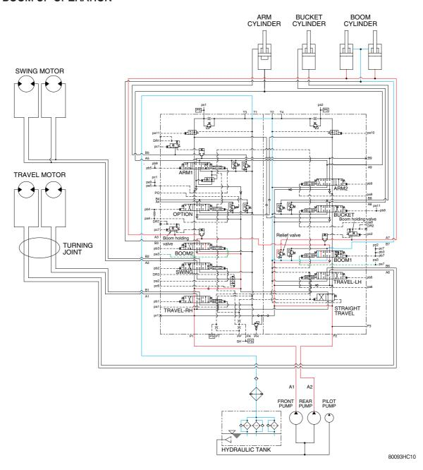
When the RH control lever is pulled back, the boom 1 and boom 2 spools in the main control valve are moved to the up position by the pilot oil pressure from the remote control valve.
