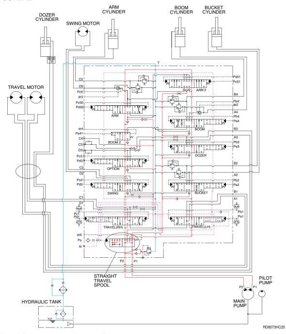
The oil from the P1 and P2 pump flows through the neutral oil passage, bypass oil passage and confluence oil passage in the main control valve. Then the oil goes to each actuator and operates them. Check valves and orifices are located on these oil passage in the main control valve. These control the oil from the main pumps so as to correspond to the operation of each actuator and smooth the combined operation.
