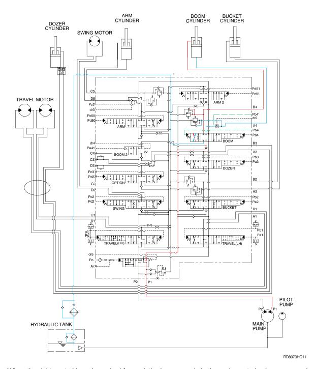
When the right control lever is pushed forward, the boom spools in the main control valve are moved to the down position by the pilot oil pressure from the remote control valve.
