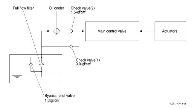
All oil returned from each actuator returns to the hydraulic tank through the control valve.
