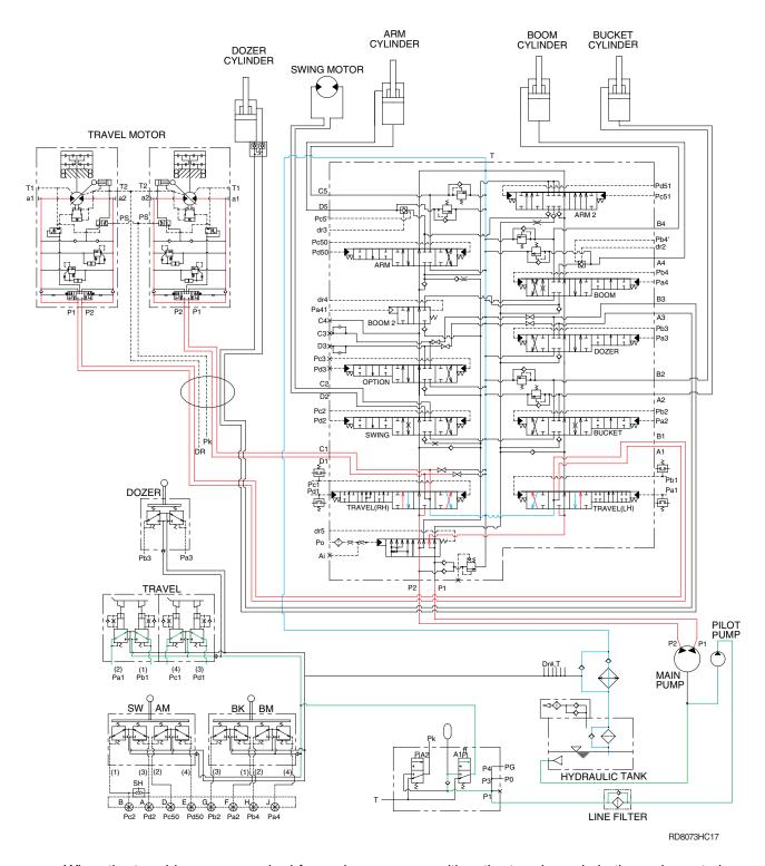
When the travel levers are pushed forward or reverse position, the travel spools in the main control valve are moved to the forward or reverse travel position by the pilot oil pressure from the remote control valve.
