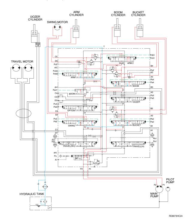
When the swing, boom, arm and bucket functions are operated, simultaneously each spool in the main control valve is moved to the functional position by the pilot oil pressure from the remote control
