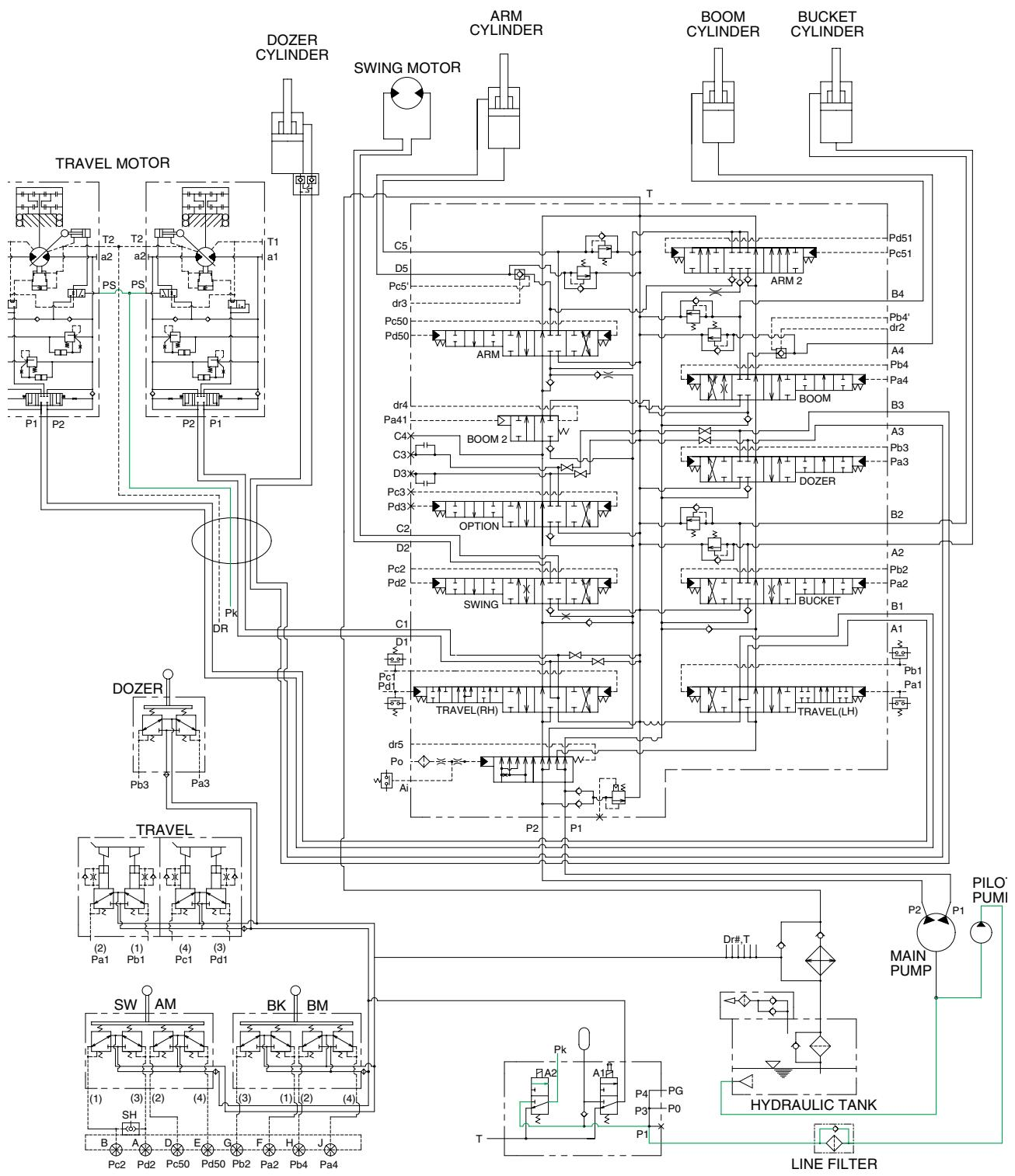
When the travel speed switch is pushed, the travel speed solenoid valve is actuated and the discharged oil from the pilot pump flows to the Pk port of pilot valve in the travel motors.
