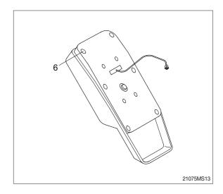
6) Install the new ROM.(Be careful of direction and assemble the cluster in the reverse order to removal).
