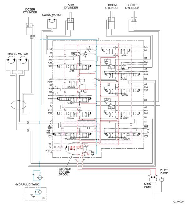
The oil from the P1 and P2 pump flows through the neutral oil passage, bypass oil passage and confluence oil passage in the main control valve. Then the oil goes to each actuator and operates them. Check valves and orifices are located on these oil passage in the main control valve. These control the oil from the main pumps so as to correspond to the operation of each actuator and smooth the combined operation.
