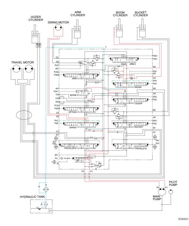
When the swing and boom functions are operated, simultaneously the swing spool and boom spools in the main control valve are moved to the functional position by the pilot oil pressure from the remote control valve.
