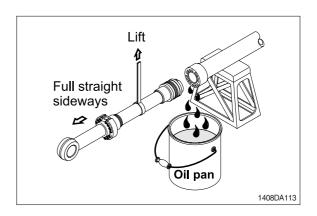
Note that the plated surface of rod assembly(2) is to be lifted. For this reason, do not use a wire sling and others that may damage it, but use a strong cloth belt or a rope.
