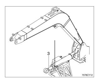
④ Disconnect boom cylinder hoses(4) and put plugs on cylinder pipe.
