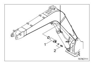
③ Lower the boom cylinder assembly(3) on a stand.
