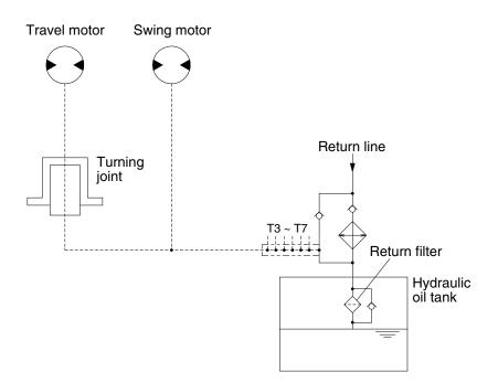
Besides internal leaks from the motors and main pump, the oil for lubrication circulates.
