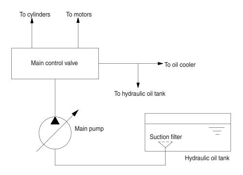
The pumps receive oil from the hydraulic tank through a suction filter. The discharged oil from the pump flows into the control valve and goes out the tank ports.
