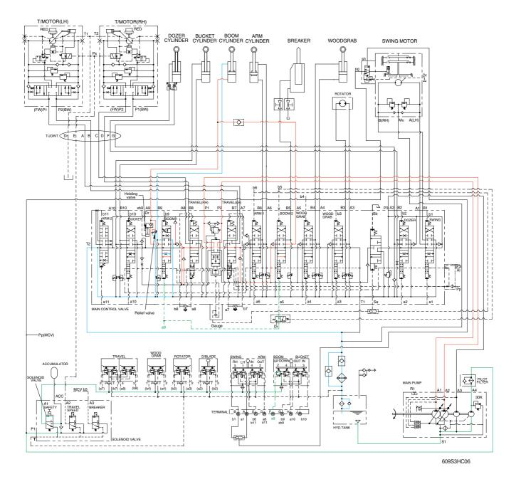
When the right control lever is pulled back, the boom spools in the main control valve are moved to the up position by the pilot oil pressure from the remote control valve.
