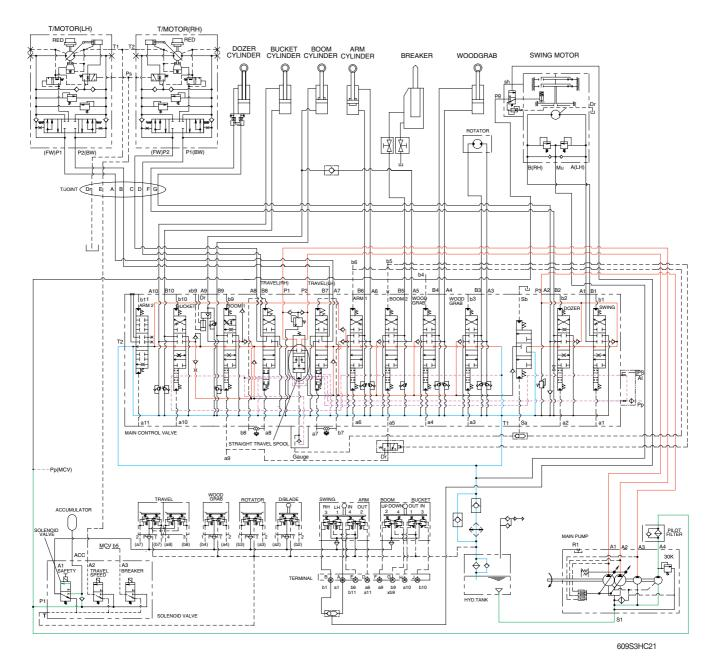
The oil from the A1, A2, A3 pump flows through the neutral oil passage, bypass oil passage and confluence oil passage in the main control valve. Then the oil goes to each actuator and operates them. Check valves and orifices are located on these oil passage in the main control valve. These control the oil from the main pumps so as to correspond to the operation of each actuator and smooth the combined operation.
