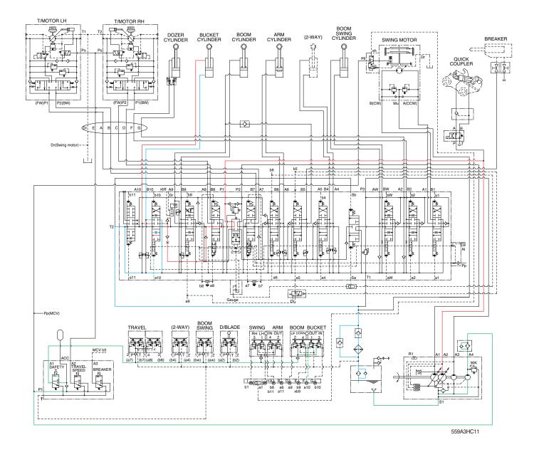
When the right control lever is pushed right, the bucket spool in the main control valve is moved to the roll out position by the pilot oil pressure from the remote control valve.
