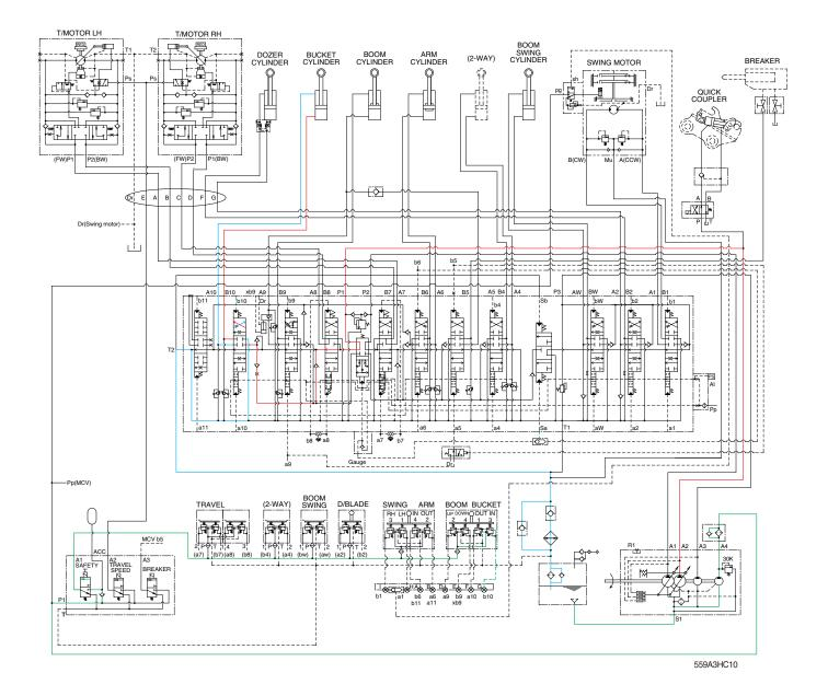
When the right control lever is pulled left, the bucket spool in the main control valve is moved to the roll in position by the pilot oil pressure from the remote control valve.
