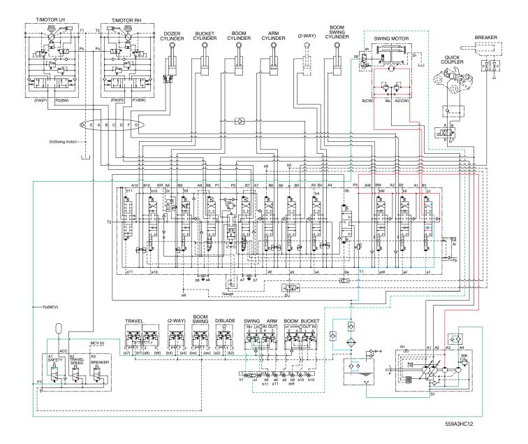
When the left control lever is pushed left or right, the swing spool in the main control valve is moved to the left or right swing position by the pilot oil pressure from the remote control valve. The oil from the A3 pump flows into the main control valve and then goes to the swing motor. At the same time, the return oil from the swing motor returns to the hydraulic oil tank through the swing spool in the main control valve. When this happens, the superstructure swings to the left or
