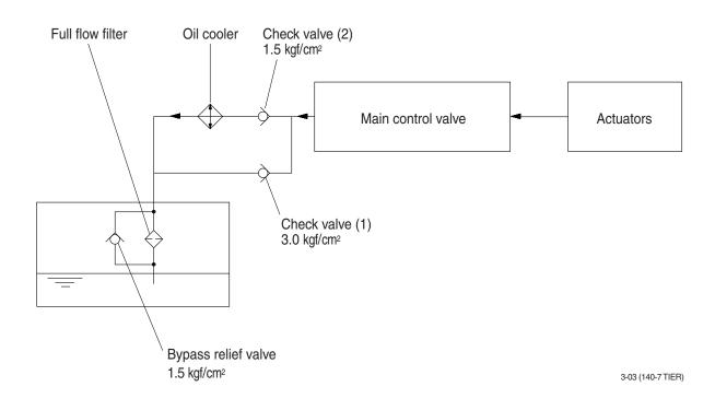
All oil returned from each actuator returns to the hydraulic tank through the control valve.
