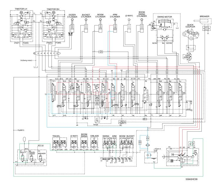
When the left control lever is pushed forward, the arm spool in the main control valve are moved to the roll out position by the pilot oil pressure from the remote control valve.
