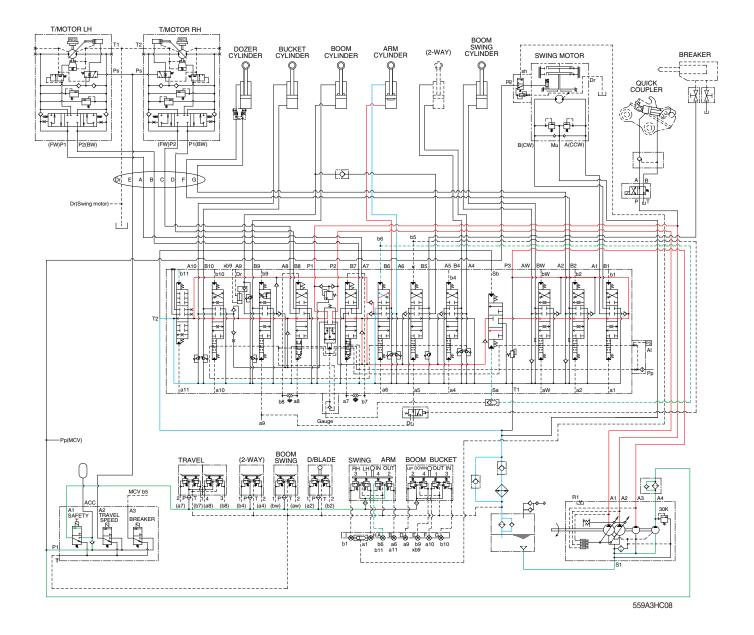
When the left control lever is pulled back, the arm spools in the main control valve are moved the to roll in position by the pilot oil pressure from the remote control valve.
