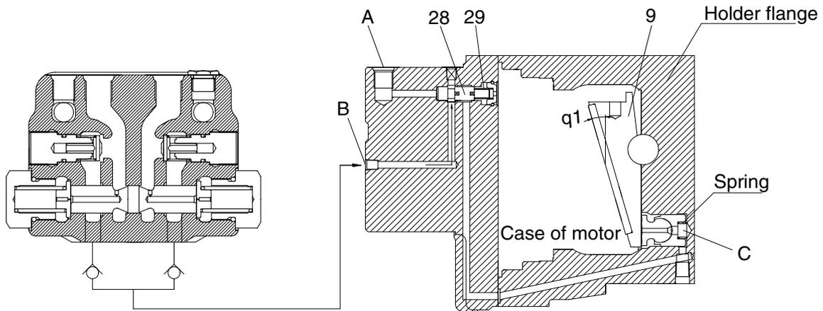
When no pilot pressure is supplied from port (A) at a pressure of 10 kgf/cm<sup>2</sup> (0.98 Mpa) or less, spool (28) is pressed toward the left by the force of spring (29), the pressurized oil supply port B is shut off, and oil in chamber (C) is released into the motor case via spool (28). Consequently, swash plate (9) is tilted at a maximum angle ( $\theta = 1^\circ$ ) and the piston displacement of hydraulic motor becomes maximum, thus leading to low-speed rotation.
