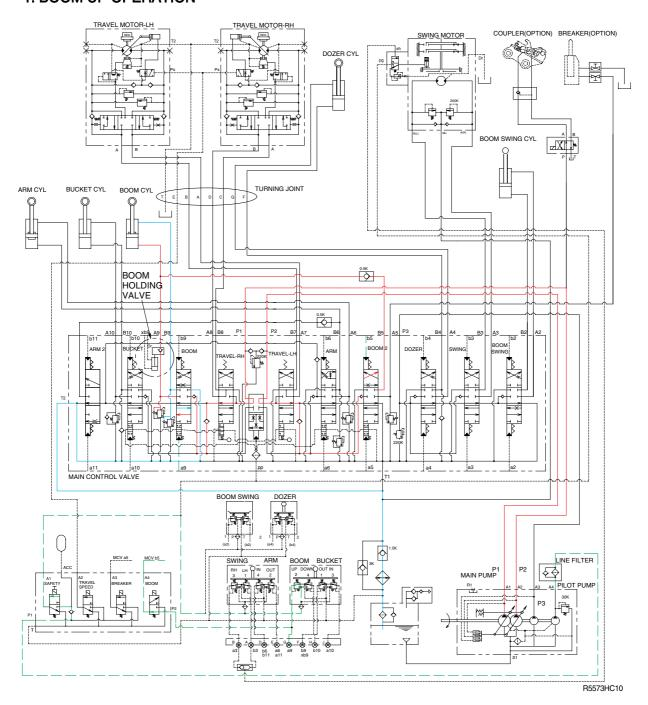
When the right control lever is pulled back, the boom spools in the main control valve are moved to the up position by the pilot oil pressure from the remote control valve.
