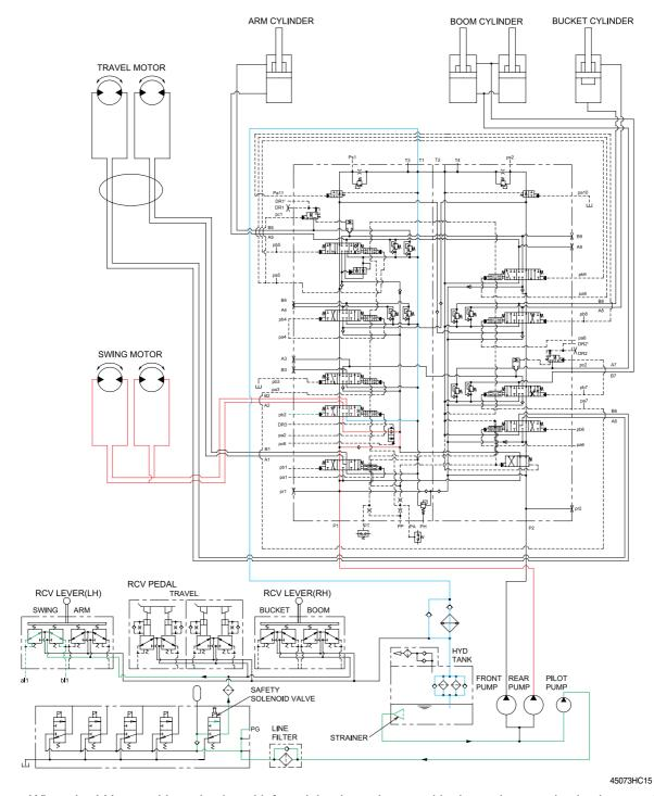
When the LH control lever is placed left or right, the swing spool in the main control valve is moved to the left or right swing position by the pilot oil pressure from the remote control valve.
