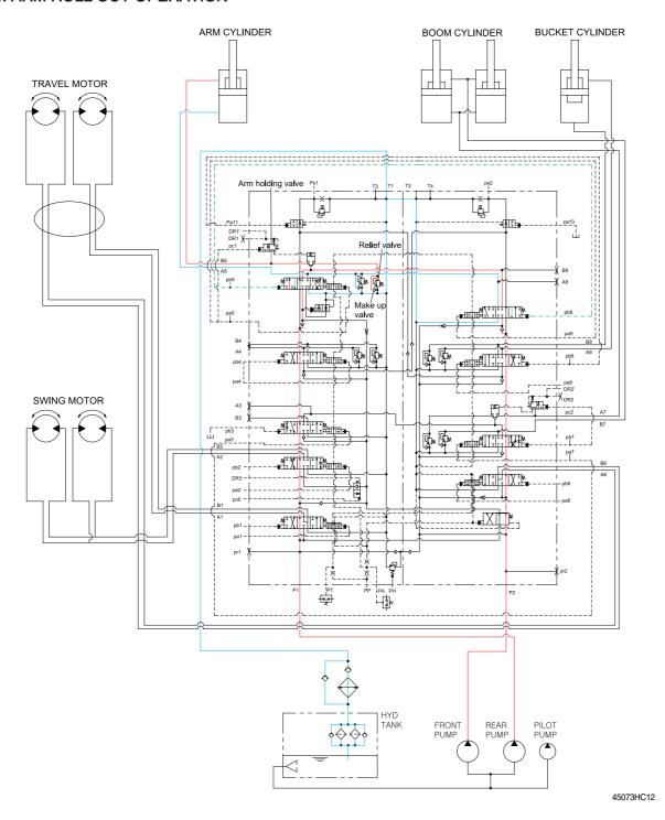
When the LH control lever is pushed forward, the arm spools in the main control valve are moved to the roll out position by the pilot oil pressure from the remote control valve. The oil from the front and rear pump flows into the main control valve and then goes to the small chamber of arm cylinder. At the same time, the oil from the large chamber of arm cylinder returns to the hydraulic oil tank through the arm spool in the main control valve.
