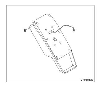
6) Install the new ROM.(Be careful of direction and assmelbe the cluster in the reverse order to removal).
