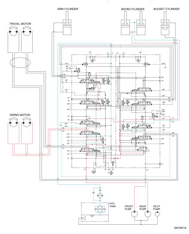
When the swing and boom functions are operated, simultaneously the swing and boom spools in the main control valve are moved to the functional position by the pilot oil pressure from the remote control valve. The oil from the rear pump flows into the swing motor through the swing spool.
