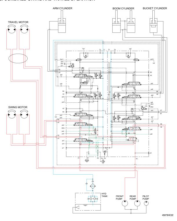
When the swing and travel functions are operated, simultaneously the swing spool and travel spools in the main control valve are moved to the functional position by the pilot oil pressure from the remote control valve. At the same time, the straight travel spool is pushed to the right by the pilot oil pressure (PP) from the pilot pump.
