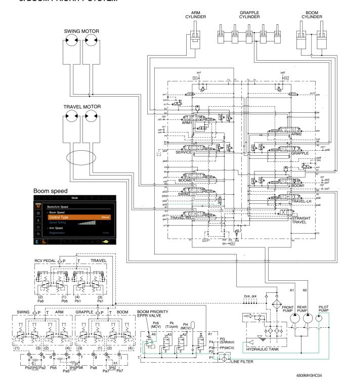
When carrying out the combined operation of swing and boom up, the boom up operating speed is lowered then normal operation.
