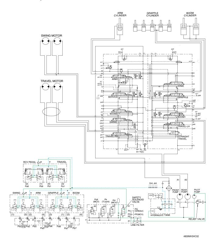
The pilot pump receive oil from the hydraulic tank. The discharged oil from the pilot pump flows to the safety solenoid valve through the line filter. The oil is filtered by the line filter.
