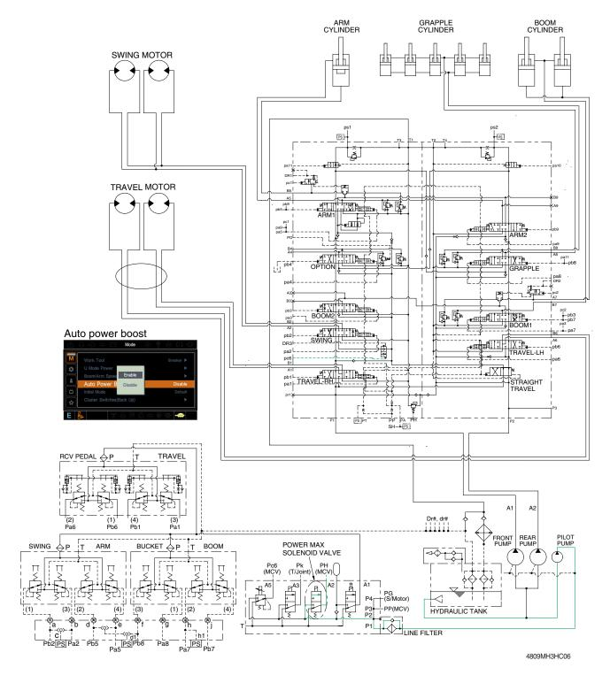
The pilot circuit consists of suction circuit, delivery circuit and return circuit.
