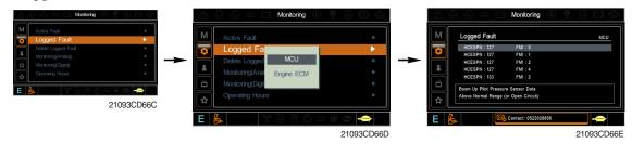
· The logged faults of the MCU or engine ECM can be checked by this menu.
