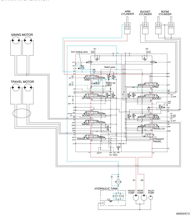
When the LH control lever is pulled back, the arm spools in the main control valve are moved the to roll in position by the pilot oil pressure from the remote control valve.
