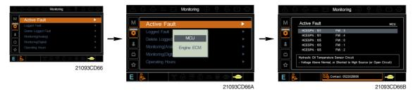
· The active faults of the MCU or engine ECM can be checked by this menu.
