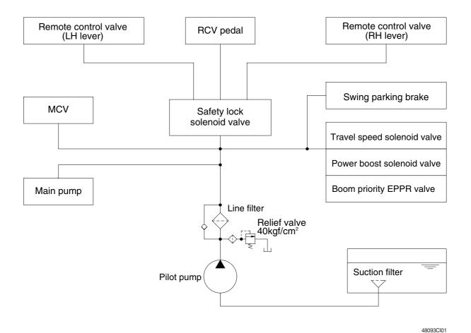
The pilot circuit consists of suction circuit, delivery circuit and return circuit.
