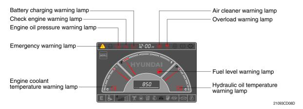
Each warning lamp on the top of the LCD pops up on the center of LCD and the buzzer sounds when the each warning is happened. The pop-up warning lamp moves to the original position and blinks when the select switch is pushed. And the buzzer stops.
