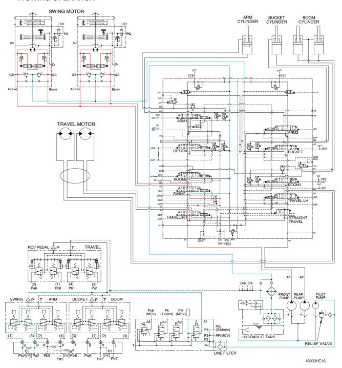
When the LH control lever is pushed left or right, the swing spool in the main control valve is moved to the left or right swing position by the pilot oil pressure from the remote control valve.
