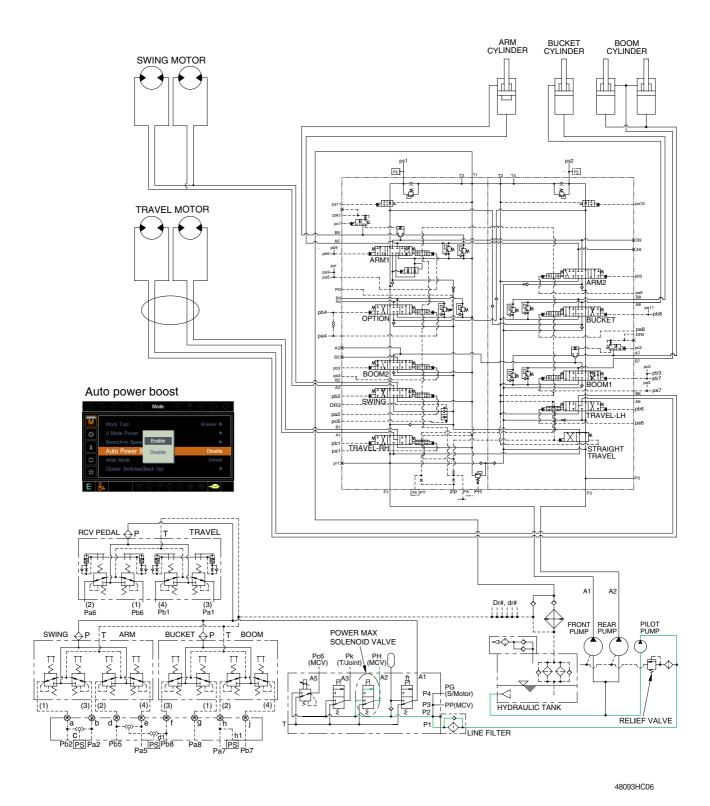
When the power max switch on the left control lever is pushed ON, the power max solenoid valve is actuated, the discharged oil from the pilot pump flow into PH port of the main relief valve of main control valve; Then the setting pressure of the main control valve is raises from 330 kgf/cm² to 360 kgf/cm² for increasing the digging power. And even when press continuously, it is canceled after 8 seconds.
