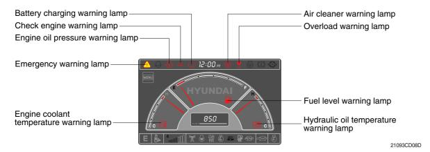
\* Each warning lamp on the top of the LCD pops up on the center of LCD and the buzzer sounds when the each warning is happened. The pop-up warning lamp moves to the original position and blinks when the select switch is pushed. And the buzzer stops. Refer to page 5-43 for the select switch.
