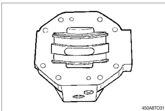
7) Visual check : Bearing areas free of scoring and no evidence of wear.
