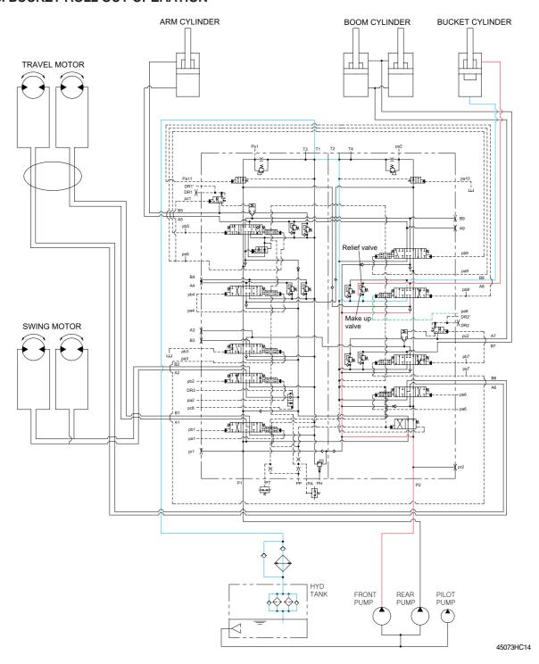
When the RH control lever is placed right, the bucket spool in the main control valve is moved to the roll out position by the pilot oil pressure from the remote control valve.
