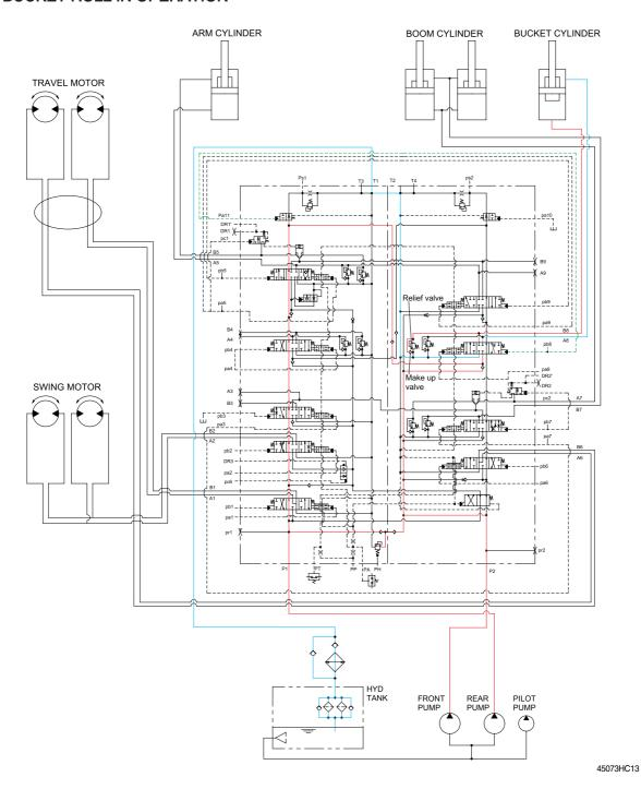
When the RH control lever is pulled left, the bucket spool in the main control valve is moved to the roll in position by the pilot oil pressure from the remote control valve.
