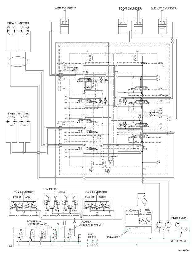
When the power max switch on the left control lever is pushed ON, the power max solenoid valve is actuated, the discharged oil from the pilot pump into Py2 port of the main relief valve of main control valve; Then the setting pressure of the main control valve is raises from 330kgf/cm² to 360kgf/cm² for increasing the digging power. And even when press continuously, it is canceled after 8 seconds.
