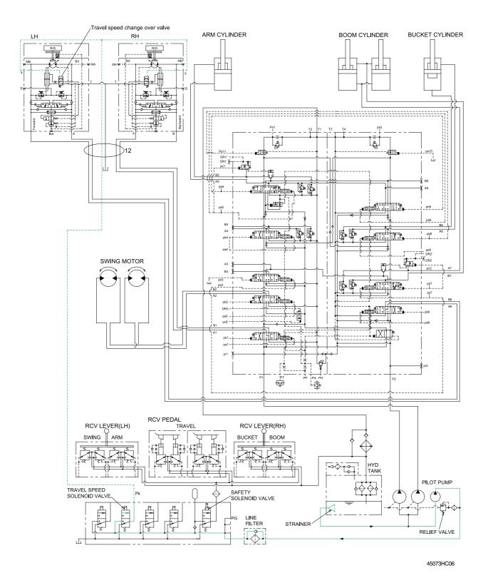
When the travel speed solenoid valve was placed in the Hi position, the pressure oil from pilot pump through line filter flows to port(Pk) of travel speed change over valve, and the control piston is pushed up, thus minimizing the displacement.
