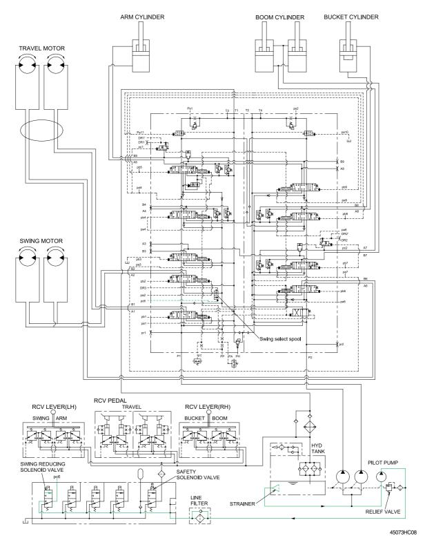
When carrying out the combined operation of swing and boom or arm, the boom or arm speed can be lowered than operating speed of swing. When the heary duty working mode in work mode is selected on the cluster, swing reducing solenoid valve actuates automatically.
