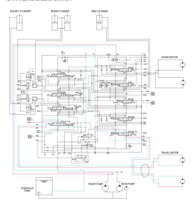
When the travel levers are pulled back, the travel spools in the main control valve are moved to the reverse travel position by the pilot oil pressure from the remote control lever.
