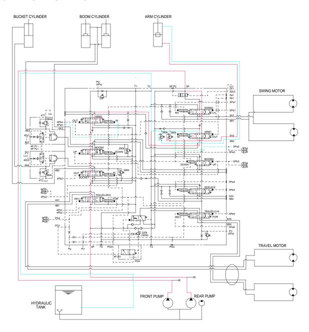
When the left control lever is pulled back, the arm spools in the main control valve are moved to the roll in position by the pilot oil pressure from the remote control valve.
