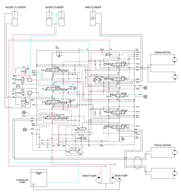
When the right control lever is pulled back, the boom spools in the main control valve are moved to the raise position by the pilot oil pressure from the remote control valve.
