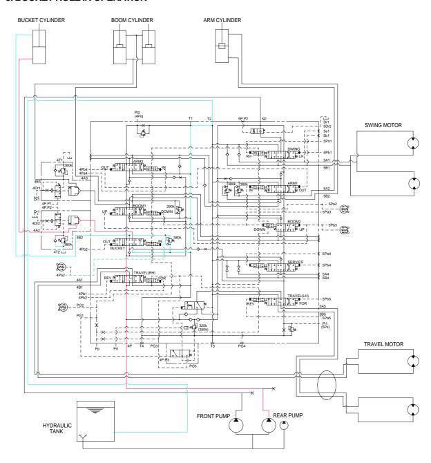
When the right control lever is pulled left, the bucket spool in the main control valve is moved to the roll in position by the pilot oil pressure from the remote control valve.
