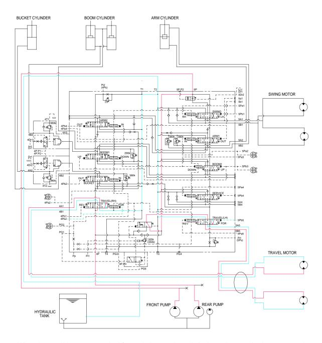
When the travel levers are pushed forward, the travel spools in the main control valve are moved to the forward travel position by the pilot oil pressure from the remote control lever.
