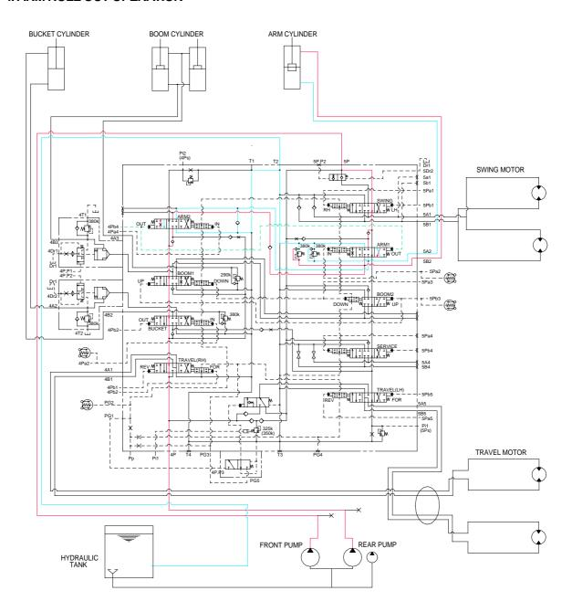
When the left control lever is pushed forward, the arm spool in the main control valve are moved to the roll out position by the pilot oil pressure from the remote control valve.
