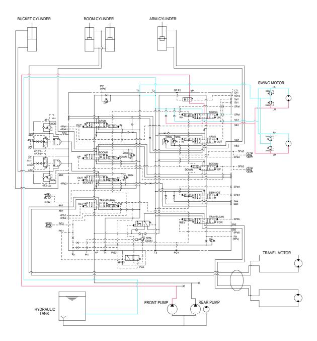
When the left control lever is pushed left, the swing spool in the main control valve is moved to the left swing position by the pilot oil pressure from the remote control lever.
