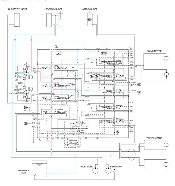
When the right control lever is pushed forward, the boom spools in the main control valve are moved to the lower position by the pilot oil pressure from the remote control valve. Also, this pilot oil flows into 4P.P1 port of boom holding valve and pushes open poppet. Then the return line open to tank port. For anti drift function of boom holding valve, see function of MCV at page 2-39.
