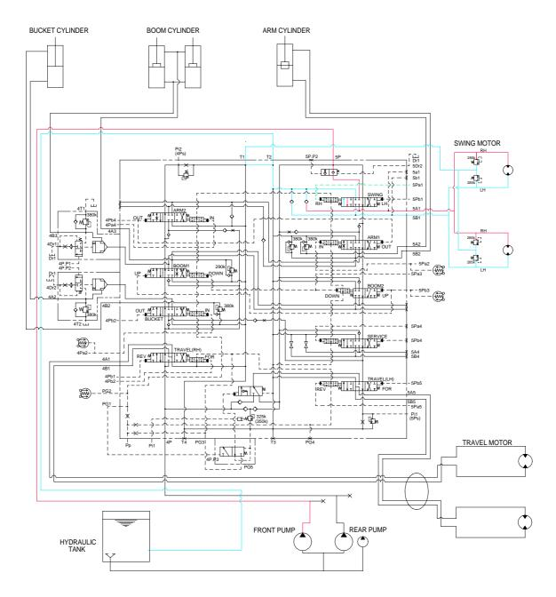
When the left control lever is pulled right, the swing spool in the main control valve is moved to the right swing position by the pilot oil pressure from the remote control lever.
