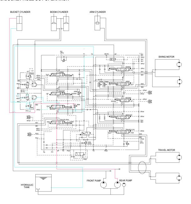
When the right control lever is pushed right, the bucket spool in the main control valve is moved to the roll out position by the pilot oil pressure from the remote control valve. Also this pilot oil flows into 4P.P2 port of bucket holding valve and pushes open poppet. Then the return line open to tank port. For anti drift function of bucket holding valve, see function of MCV at page 2-39.
