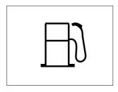
① This lamp lights on when fuel level is below 50  $\it l$  . In that case, replenish oil.
