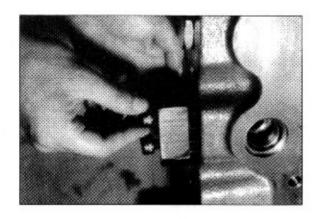
③ Mount flange cap (75) attached O-ring (76) to tank port and tighten socket head bolt (78).
