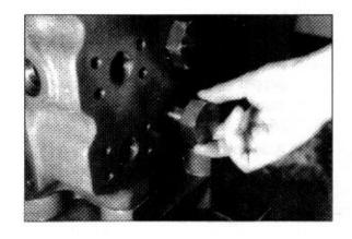
Insert sleeve (59) into LH travel part and assemble plug (42) attached O-ring (43).
