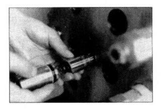
4 Assemble plug (51) attached O-ring (49) and backup ring (50) into arm 5A2 port.
