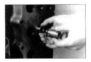
③ Assemble poppet (57), spring (41), Oring (49), backup ring (50) and plug (58) into bucket 4A2 port.
