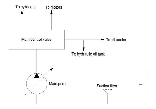
The pump receive oil from the hydraulic tank through a suction filter. The discharged oil from the pump flows into the control valve and goes out the tank ports.
