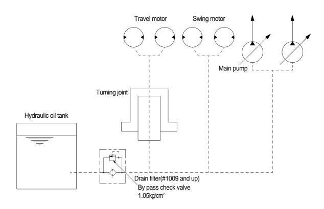
Besides internal leaks from the motors and main pump, the oil for lubrication circulates. These oil have to be fed to the hydraulic tank through drain filter.
