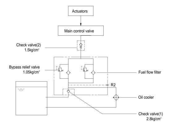
All the oil returned from each actuator returns to the hydraulic tank through the control valve.
