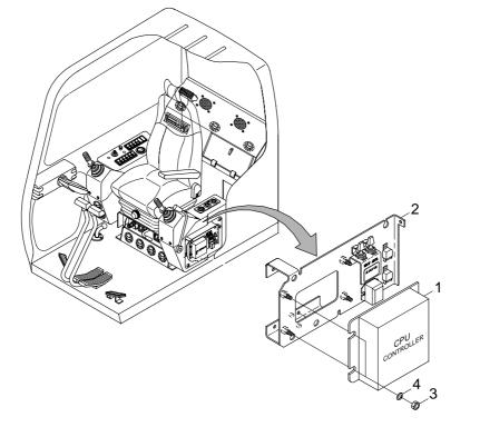
1 CPU controller 2 Controller mounting bracket 3 Nut 4 Spring washer
