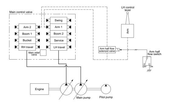
When arm half flow switch is turned ON, the arm half flow solenoid value is switched to ON and it cancels the junction of the oil flow from two pumps.
