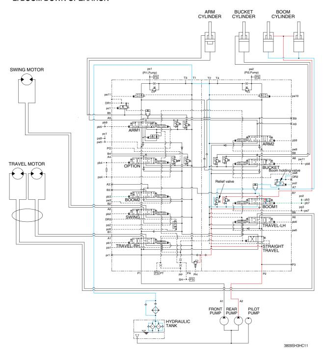
When the RH control lever is pushed forward, the boom 1 spools in the main control valve are moved to the down position by the pilot oil pressure from the remote control valve.
