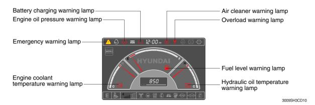
Each warning lamp on the top of the LCD pops up on the center of LCD and the buzzer sounds when the each warning is happened. The pop-up warning lamp moves to the original position and blinks when the select switch is pushed. And the buzzer stops. Refer to page 5-49 for the select switch.
