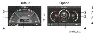
1 Engine coolant temperature gauge
