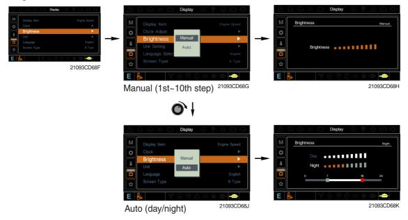
If "Auto" is chosen, brightness for day and night can be differently set up. Also by using the bar in lower side, users can define which time interval belongs to day and night. (in bar figure, gray area represents night time while white shows day time)
