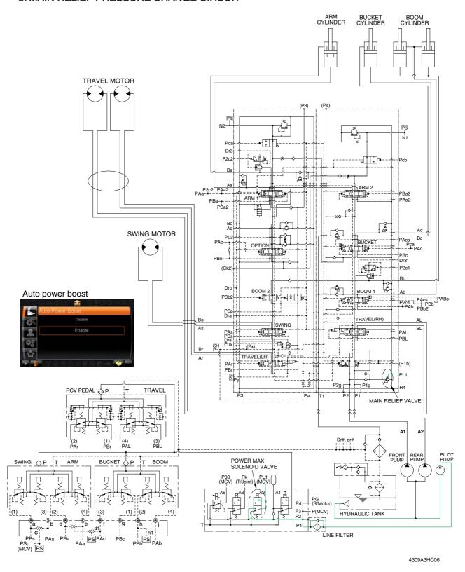
When the power max switch on the left control lever is pushed ON, the power max solenoid valve is actuated, the discharged oil from the pilot pump flow into PL1 port of the main relief valve of main control valve; Then the setting pressure of the main control valve is raises from 330 kgf/cm² to 360 kgf/cm² for increasing the digging power. And even when press continuously, it is canceled after 8 seconds.
