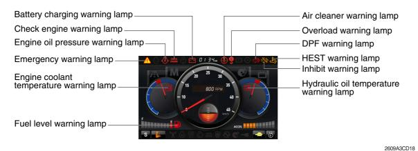
\* Each warning lamp on the top of the LCD pops up on the center of LCD and the buzzer sounds when the each warning is happened. The pop-up warning lamp moves to the inal position and blinks when the select switch is pushed. And the buzzer stops. Refer to page 5-58 for the select switch.
