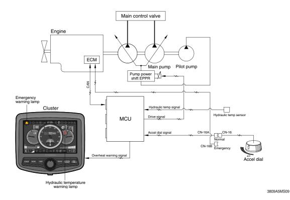
1. The engine coolant temperature or the hydraulic oil temperature is overheated over 100°C, the warning lamp is ON and the pump input torque or the engine speed is reduced as below logic table.
