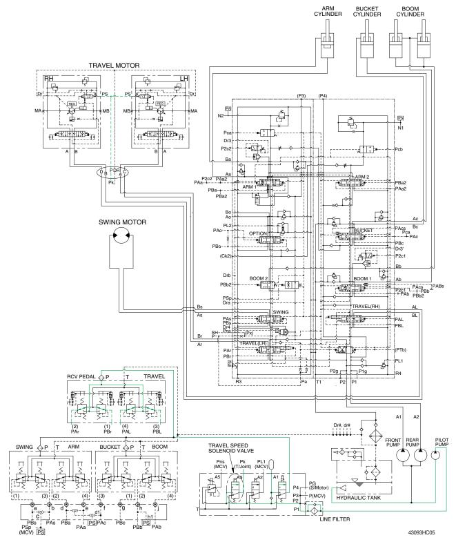
When the travel speed switch is pushed, the travel speed solenoid valve is actuated and the discharged oil from the pilot pump flows to the **Pi** port of pilot valve in the travel motors.
