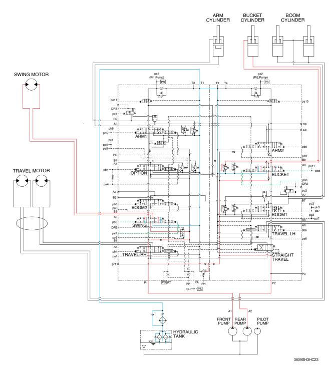
When the swing and bucket functions are operated, simultaneously the swing spool and bucket spool in the main control valve are moved to the functional position by the pilot oil pressure from the remote control valve.
