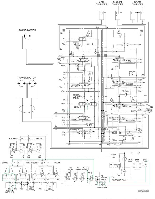
When carrying out the combined operation of swing and arm of the left control valve, the swing speed can be lowered than operating speed of arm.
