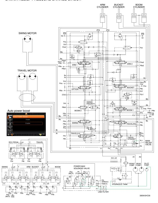
When the power max switch on the left control lever is pushed ON, the power max solenoid valve is actuated, the discharged oil from the pilot pump flow into PL1 port of the main relief valve of main control valve; Then the setting pressure of the main control valve is raises from 330 kgf/cm² to 360 kgf/cm² for increasing the digging power. And even when press continuously, it is canceled after 8 seconds.
