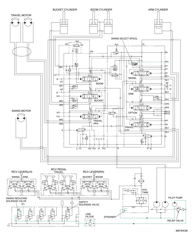
When carrying out the combined operation of swing and boom or arm, the boom or arm speed can be lowered than operating speed of swing. When the heary duty working mode in work mode is selected on the cluster, swing reducing solenoid valve actuates automatically.
