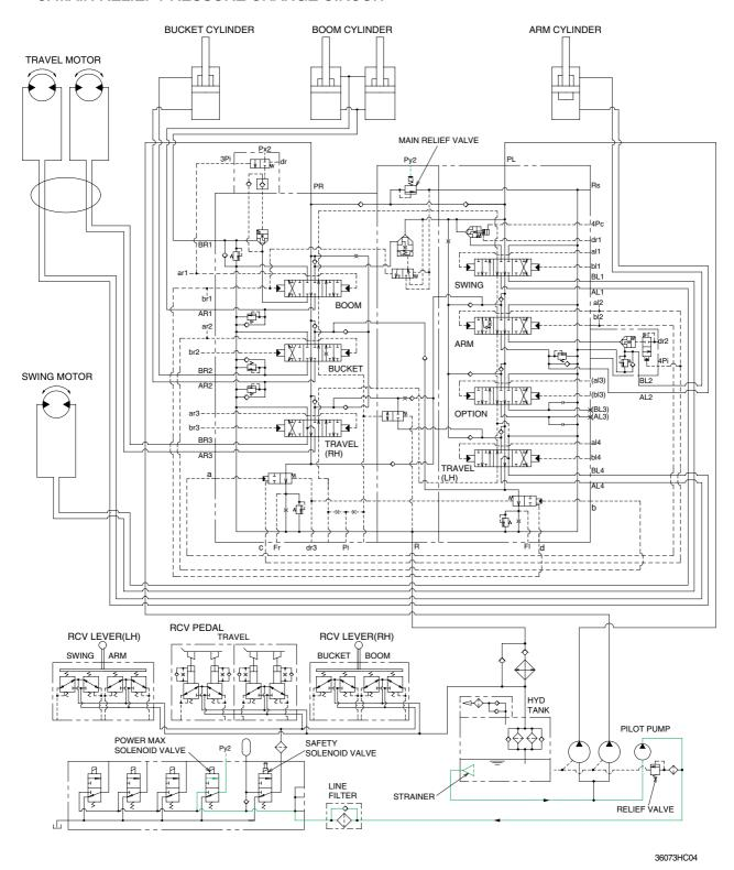
When the power max switch on the left control lever is pushed ON, the power max solenoid valve is actuated, the discharged oil from the pilot pump into Py2 port of the main relief valve of main control valve; then the setting pressure of the main control valve is raises from 330kgf/cm² to 360kgf/cm² for increasing the digging power. And even when pressed continuously, it is canceled after 8 seconds.
